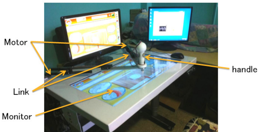
Fig. 1 2D robotic rehabilitation system of upper limb for stroke patients.
